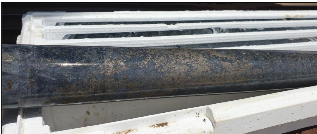
Photograph 2 – Intersection of NPDD013 at 578.4m showing matrix to semi-massive sulphides (Po- Pn-Cpy)
