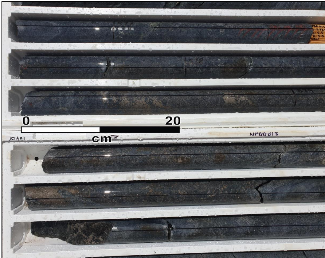
Photograph 1 – Intersection of NPDD013 from 576.8m to 581.5m showing matrix and heavy disseminated sulphides (Po-Pn-Cpy)
